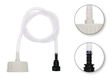
Warm the 30mm hose until pliable and insert the 8mm hose barb (green connector) and insert the 10mm hose barb (black connector) on the opposite side.
